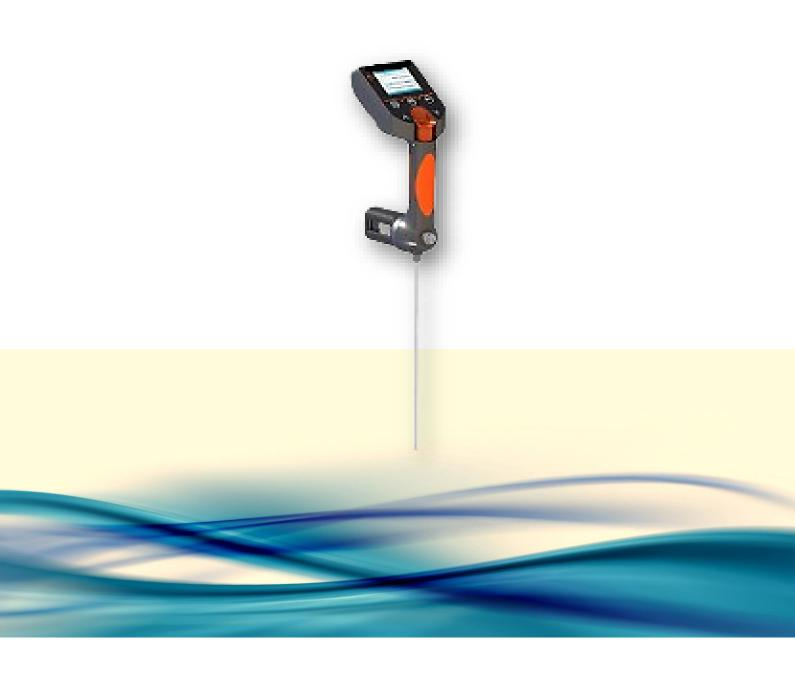
Portable Density Meter LD-LPDM-A10 measures 0 g/cm<sup>3</sup> to 3.0 g/cm<sup>3</sup> density at a temperature range from 5°C to 55°C suitable for a wide spectrum of liquids in variable temperatures. Our meter offers quick and efficient results with a minimum of 2ml samples. It is capable of converting into standard density, concentration, and specific gravity at the same time.
